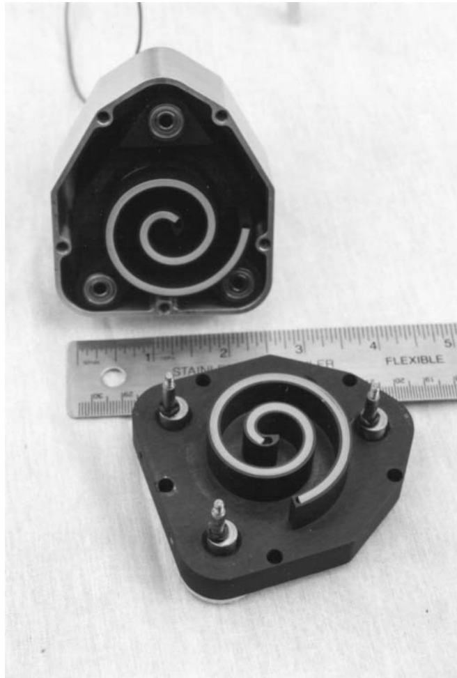
FIGURE 12.4 Typical scroll showing idler shafts.
