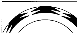
FIGURE 16.17 Bi-directional grooved seal face (John Crane Inc.).
