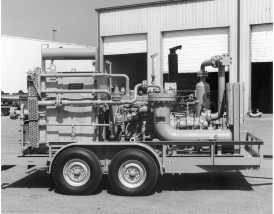
FIGURE 23.10 Trailer-mounted CAT G3304NA/C12 sulfur unit.
